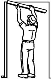
3. Slip head over wall and engage head aligning tab in slot of hinge jamb.
