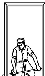
8. Size opening by inserting wood spreader cut to exact opening width and fasten sill anchor at strike jamb with nails or screws.
