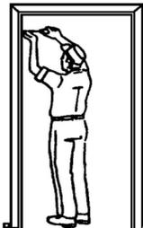
5. Position adjustable pressure anchor by turning adjusting screw clockwise an equal amount for both anchors. After contact is made with studs, continue tightening until frame is wedged between studs. (Do not over-tighten.)
